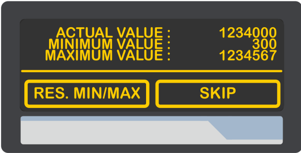
Display with minimum and maximum value
