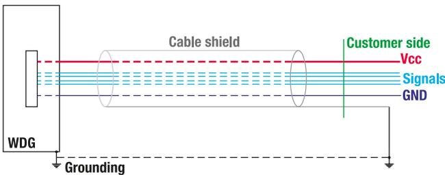
L2/L3, T3: Cable shield connected to encoder housing.
