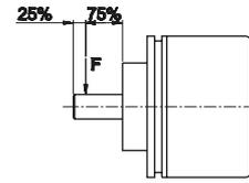
The bearings are treated with a special grease able to withstand extreme temperatures, high speeds and loads, as well as constant operation in reverse. The grease remains stable over a long period of time. The indicated radial-bearing load relates to the point F of the applied force. The useful life of the bearings is stated in the number of revolutions. The life can be converted into hours using the following formula:
