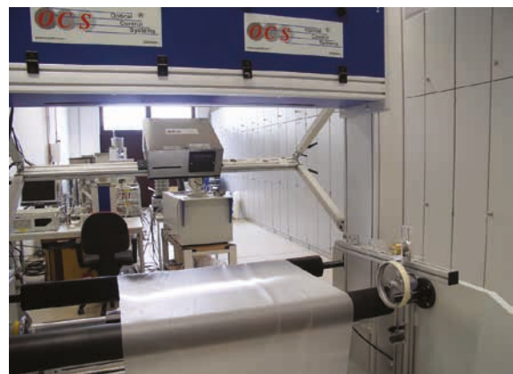
Image 2 For transparent materials they use transmitted light
