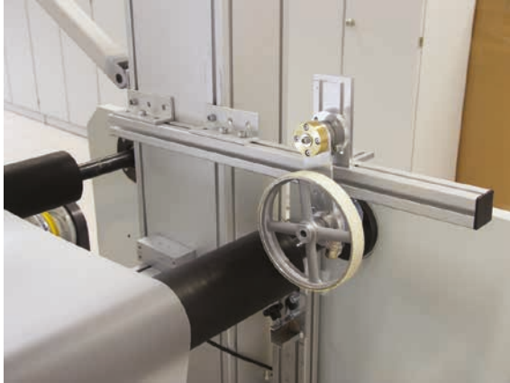
Image 4 The encoder can easily be mounted with the spring lever
