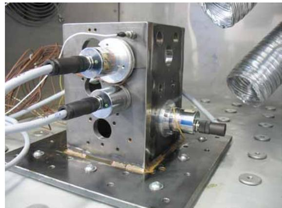
After that, a temperature change test is run for five cycles with the determined operating limits (LOL and UOL) for the rapid thermal transitions stress test. The temperature change occurs at at least 50 K/min. The temperature is maintained for a determined period of time for the UOL and LOL.
