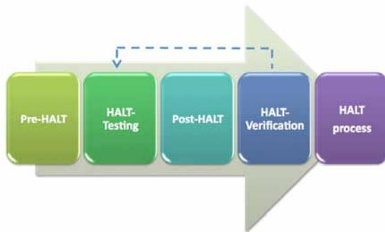
Pre-HALT is the preparations needed for the test (such as defining error criteria, creating function tests). The actual tests are run during HALT testing. The HALT test results are then analysed in the post-HALT phase and optionally a redesign is performed. The HALT testing is then run once again for the redesigned sample to verify the results.
