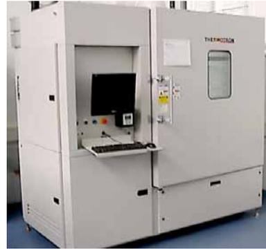
The AST chamber's test air is heated by an electrical heater to max. 200 °C. The LN2 system (induction of liquid nitrogen) cools the chamber enabling rapid temperature changes. The vibration is created by pneumatic cylinders which impact the test bed from below.
