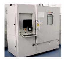
The AST chamber's test air is heated by an electrical heater to max. 200 °C. The LN2 system (induction of liquid nitrogen) cools the chamber enabling rapid temperature changes. The vibration is created by pneumatic cylinders which impact the test bed from below.
