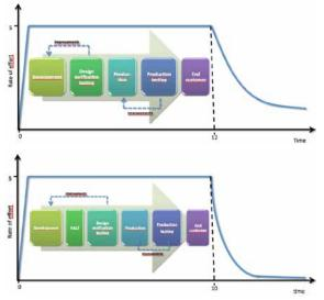
If we observe the level of reliability compared with the failure rate  $\lambda$ , we can see that the HALT test shifts the bathtub curve downwards during the usage phase, which indicates that the failure rate has fallen.
