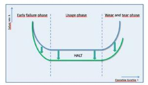
According to the Arrhenius equation, the rule of thumb (for electronics): A temperature increase of 10  $^\circ C$  doubles the failure rate.
