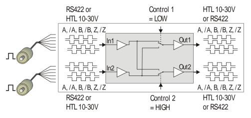
Both inputs can be individually set to either symmetric (differential) format using A, /A, B, /B, Z, /Z channels, or to asymmetric (single-ended) format using A, B, Z channels only. Acceptable input levels are RS422, TTL and HTL 10 ... 30 V.
