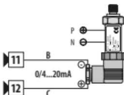
For signals 0/4..20mA with **external power of sensor**
