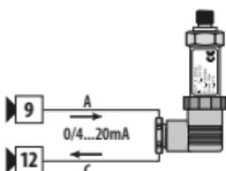
For signals 0/4..20mA with **two-wire sensor**
