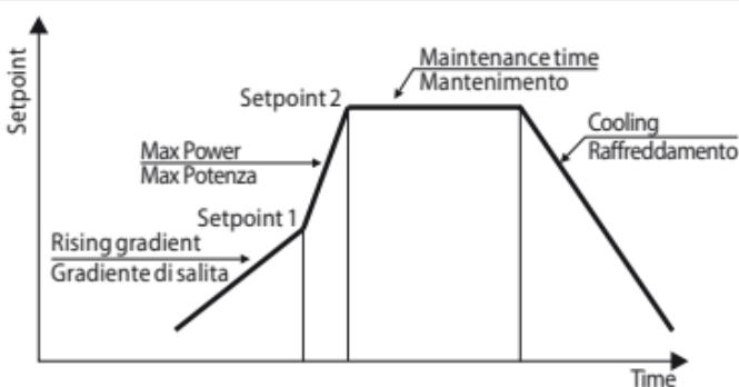
Cycle starts at each activation of the controller, or via digital input if it is enabled for this type of functioning (parameters 94 d.1.IF, or 101 d.12.F set as 5E./5E. or RUN).
