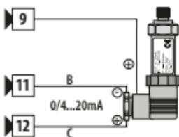
For signals 0/4..20mA with **three-wire sensor**
